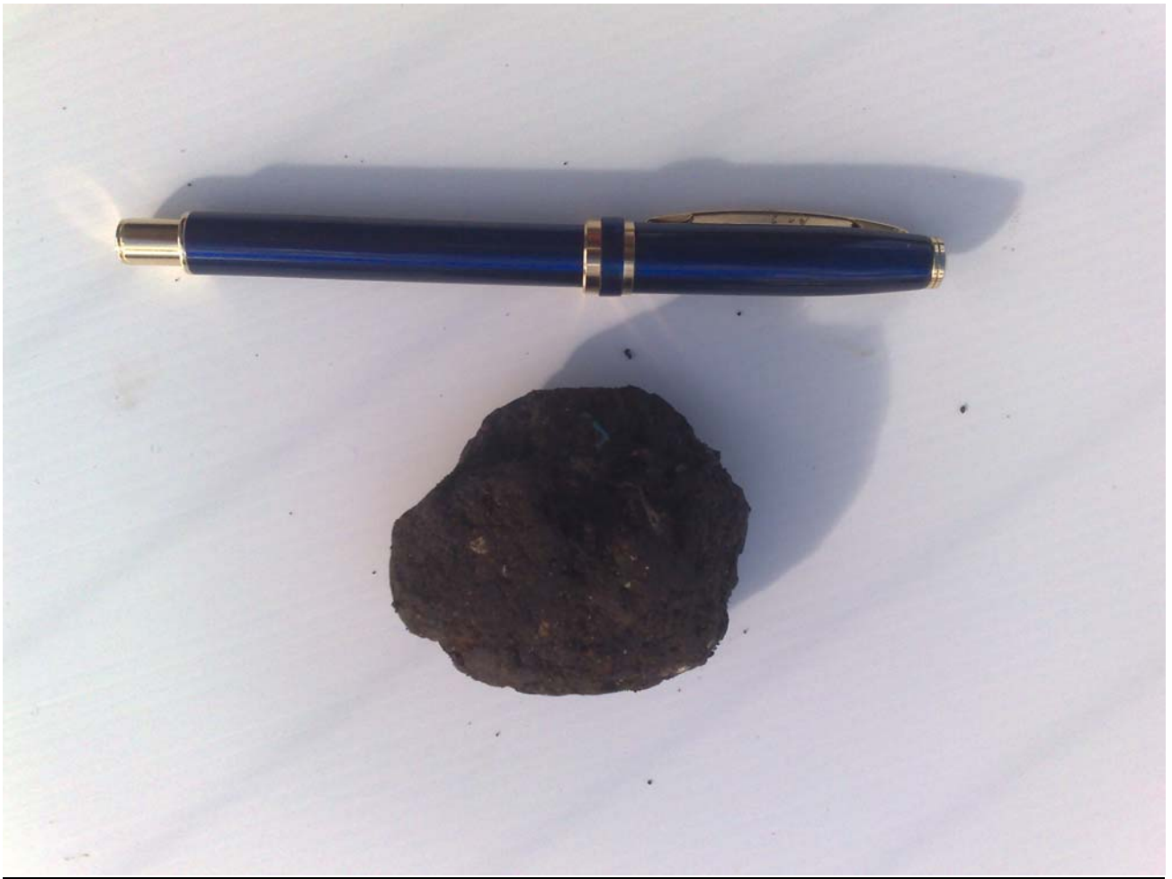
2. Mildly radioactive rock, detected at and removed from the waste sorter
